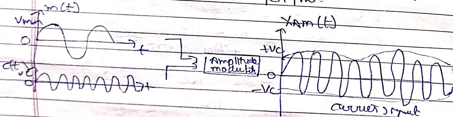
(ii) AM radio transmitter radiator, 6 kW power when modulation % is 70%. Determine the carrier power.
